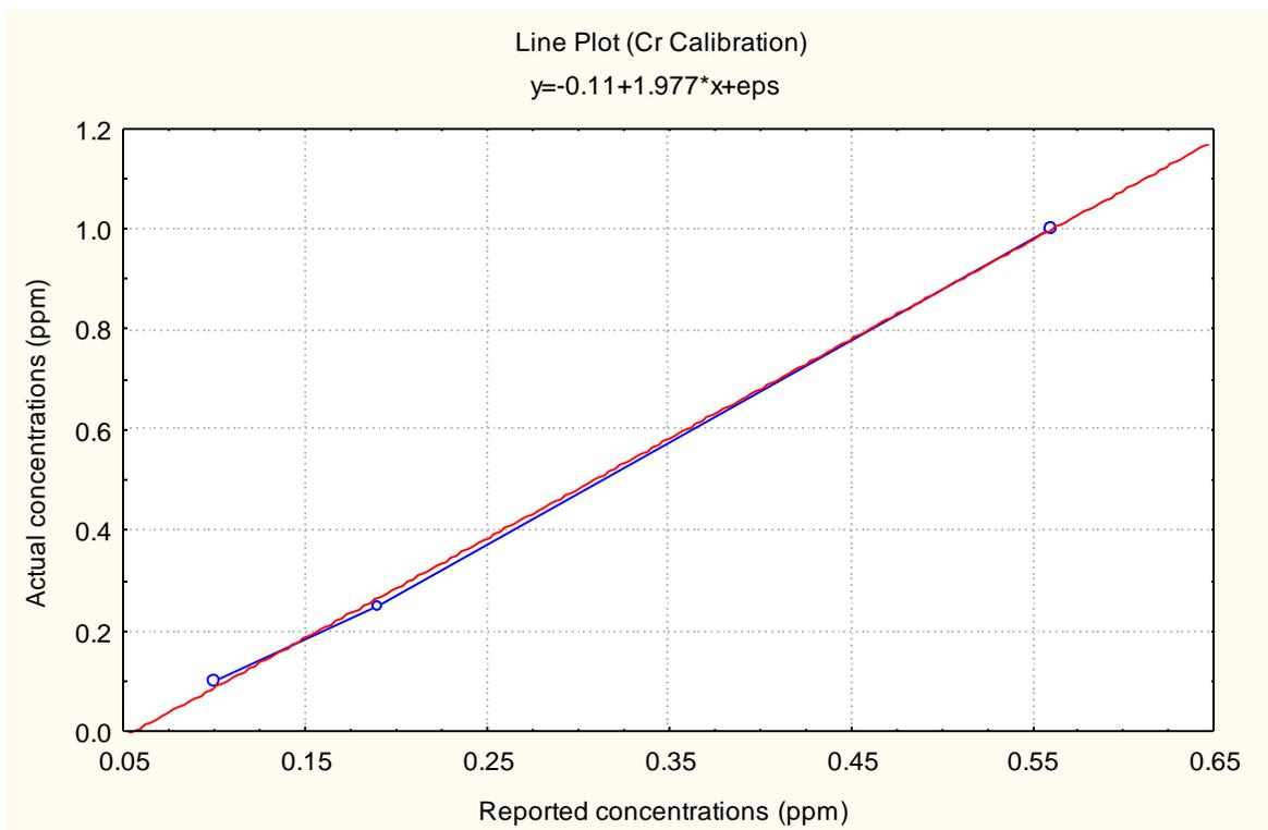
Figure 2: A typical Calibration curve for Cr for analyses by FAAS by one laboratory
