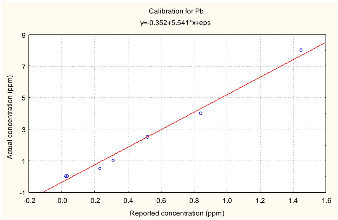
Figure 1: A typical Calibration curve for Pb for analyses by FAAS by one laboratory
