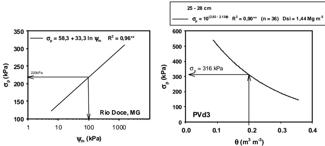
Figure 2: Estimation of the maximum pressure that should be applied to the soil in order to avoid soil compaction using the Load Bearing Capacity model.
