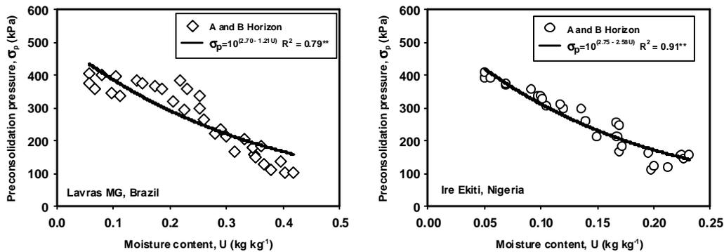
Figure 4: Representative Load Bearing Capacity Model for both Site following Homogeneity test.
