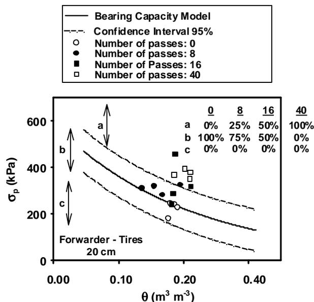
Figure 6: Assessment of the effect of different No of passes of Forwarder with tires on precompression stress of a Yellow Ultisols using Load Bearing Capacity model
