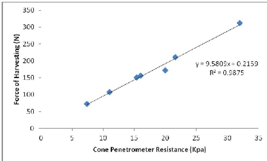
**Fig. 5.** Relationship between force of harvesting and cone penetrometer resistance on a soil planted to groundnut
