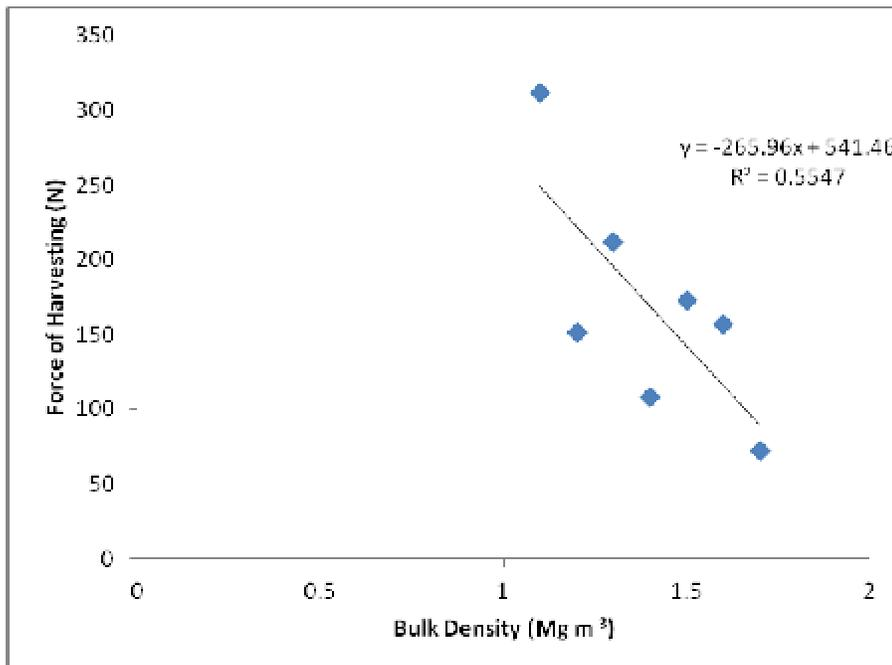
**Fig. 6.** Relationship between force of harvesting and soil bulk density on a soil planted to groundnut
